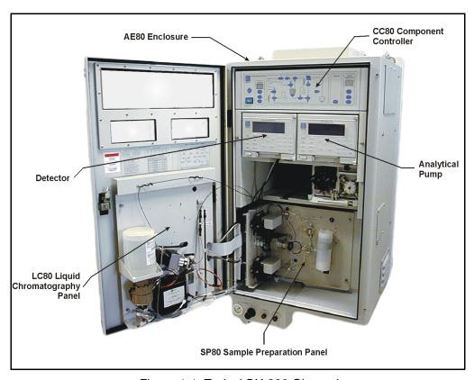
Figure 1-1. Typical DX-800 Channel
