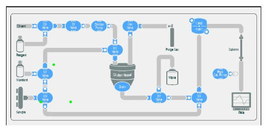
Figure 4-3. CC83 Front Panel: SP83 for Dilution with Reagent Addition
