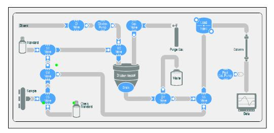
Figure 4-2. CC82 Front Panel: SP82 for Dilution or Direct Injection
