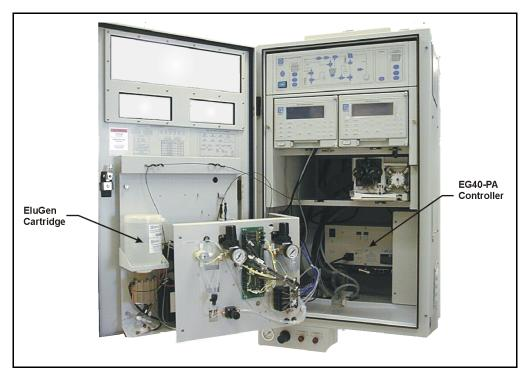
Figure 6-2. DX-800 with EG40-PA Installed
