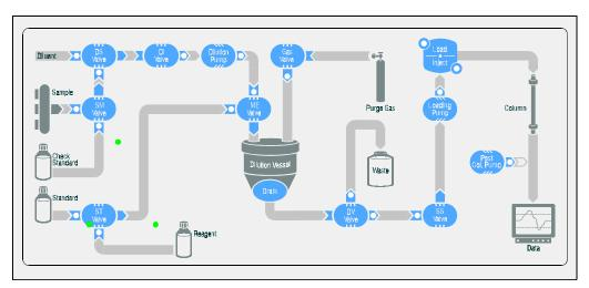
Figure 4-4. CC84 Front Panel: SP84 for Concentration with Reagent Addition
