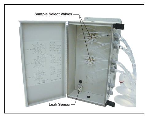
Figure 8-1. SS80 with Two Sample Valves
