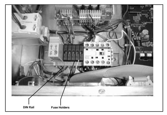
Figure 11-2. Changing a CC80 Fuse CC80 Top Cover Removed—Top View
