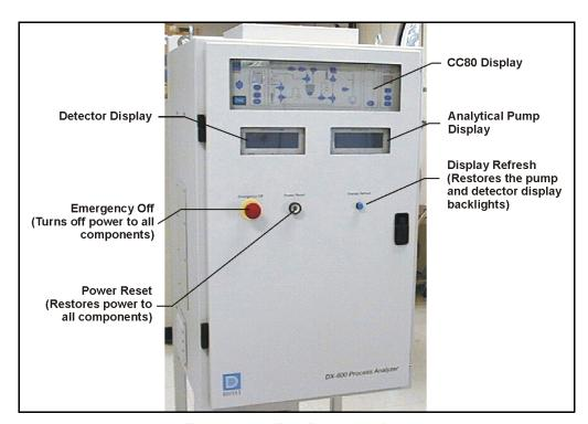
Figure 2-1. AE80 Enclosure Door
