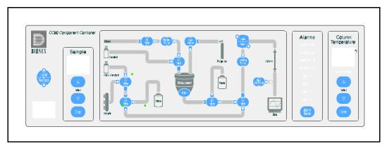
Figure 3-1. CC81/SP81 Front Panel (for Concentration)
