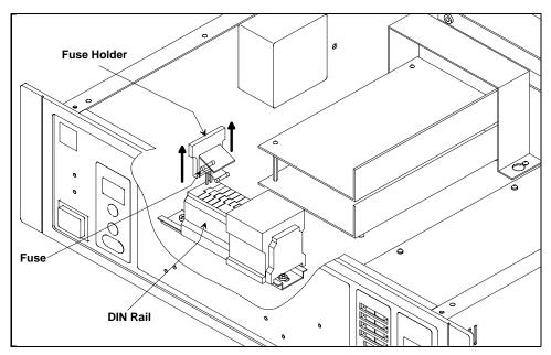
Figure 11-3. Changing a CC80 Fuse CC80 Top Cover Removed--Cutout View
