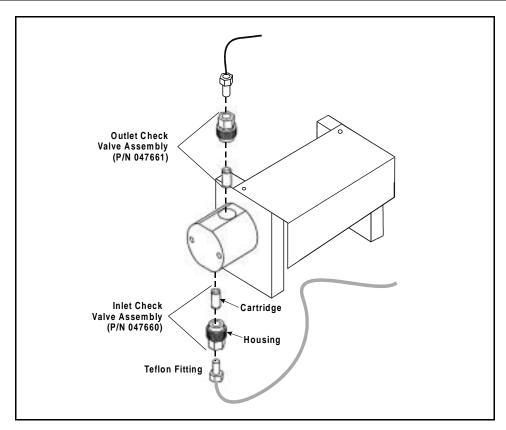
Figure 11-1. Precision Displacement Pump Check Valves
