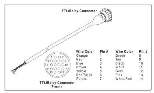
Figure 12-4. TTL/Relay Cable and Connector Pinout
