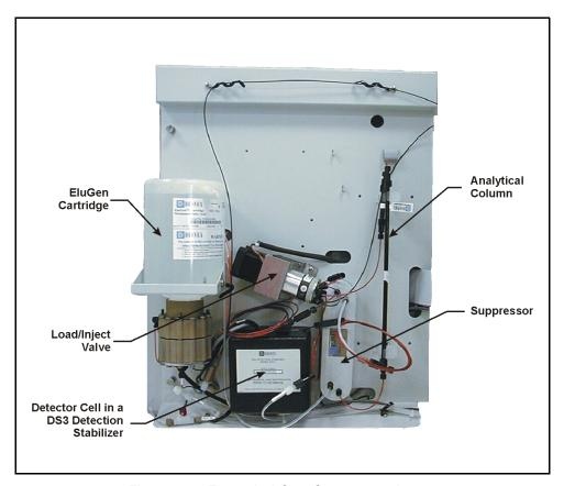
Figure 5-1. Example LC80 Component Layout
